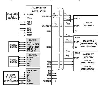
Figure 2. ADSP-2181/ADSP-2183 Basic System Configuration
